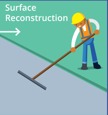
Surface Reconstruction Top concrete layer removed, rebar installed and new concrete surface added.
