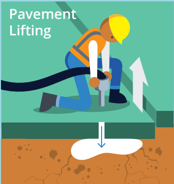
Pavement Lifting Material is injected into sunken street segments to raise them up.
