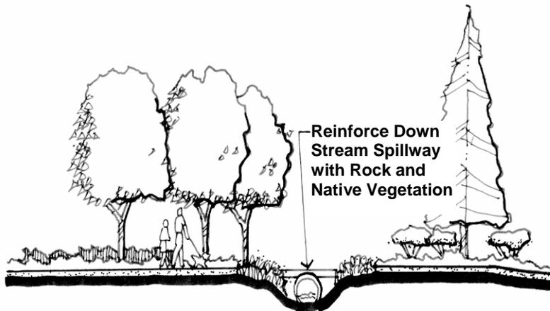
**Figure 13.** *Low Water Crossing of Minor Stream or Drainage*
