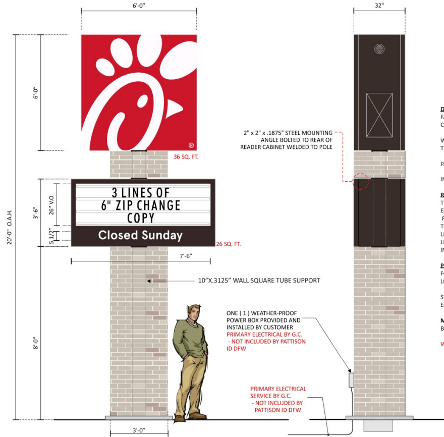
OPTION 2 A D/F PYLON WITH READERBOARD SIGN ONE (1) REQUIRED - MANUFACTURE AND INSTALL
